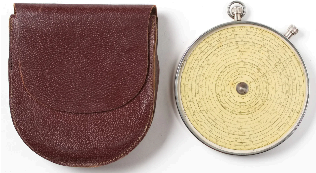
A Fowler Long Scale Circular slide rule, sometimes also called the Magnum. It is controlled by the two knobs on its edge. Sphere Research Corporation
