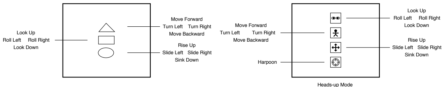
32: Two possible “virtual joystick” navigation elements. The left diagram depicts the widgets used in the DIVE environment. The right depicts “heads-up” mode in VRweb.
